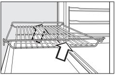
When pushing the rack back in, always ensure that the safety notches are at the rear of the oven (see illustration).
